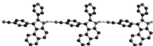
Figure 2. Part of the hydrogen-bonded chain present in crystals of 3 . The chain extends along the b axis with successive molecules related by a unit cell translation. All chains in the crystal are chiral and are of the same handedness.
